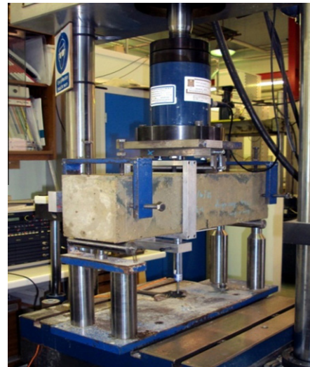
Fig. 4. Three point load (flexural strength) test underway.
