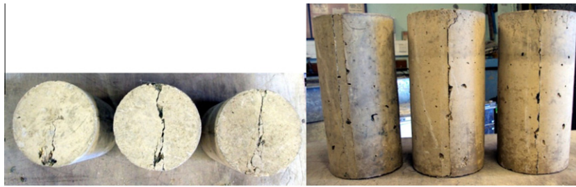
Fig. 11. Tested samples for splitting tensile strength at 28 days.
