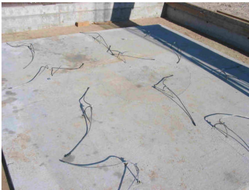
Fig. D.11 Crack line on the concrete test n°1
