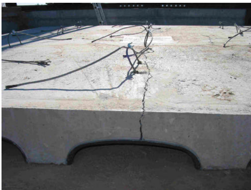
Fig. D.12 Crack line detail on the concrete test n°1
