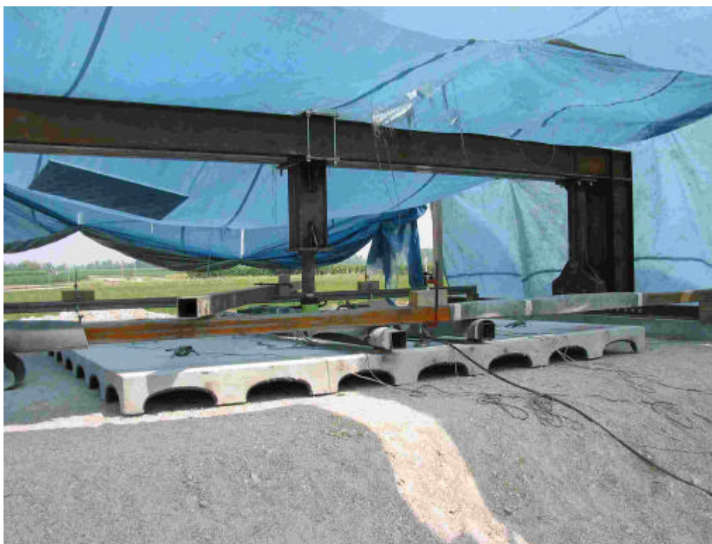
Fig. D.22 Concrete test n°11 on gravel subgrade
